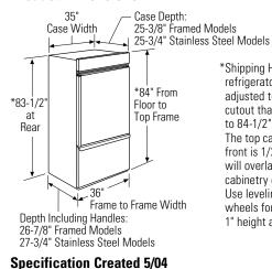
\*Shipping Height. The refrigerator can be adjusted to fit into a cutout that is 83-1/2" min. to 84-1/2" max. height. The top case trim at the front is 1/2" higher and will overlap upper cabinetry or soffit. Use leveling legs and wheels for a maximum 1" height adjustment.
